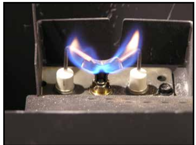
Figure 3.1 IPI Pilot Flame Patterns
