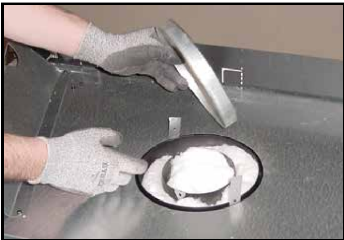
Figure 9.3 Remove the seal cap.
