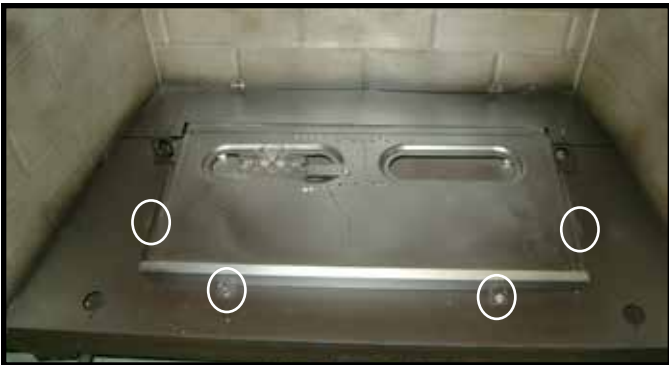
Figure 3.9 Remove Burner Skirt
